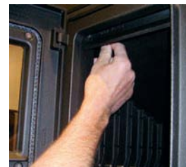
Im. 4: Losening the retaining plate
